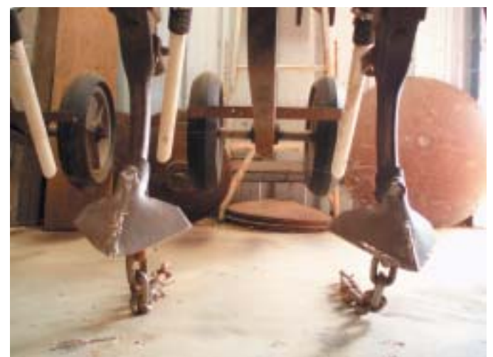
A 28 run combine fitted with wide but steep points for furrow sowing
