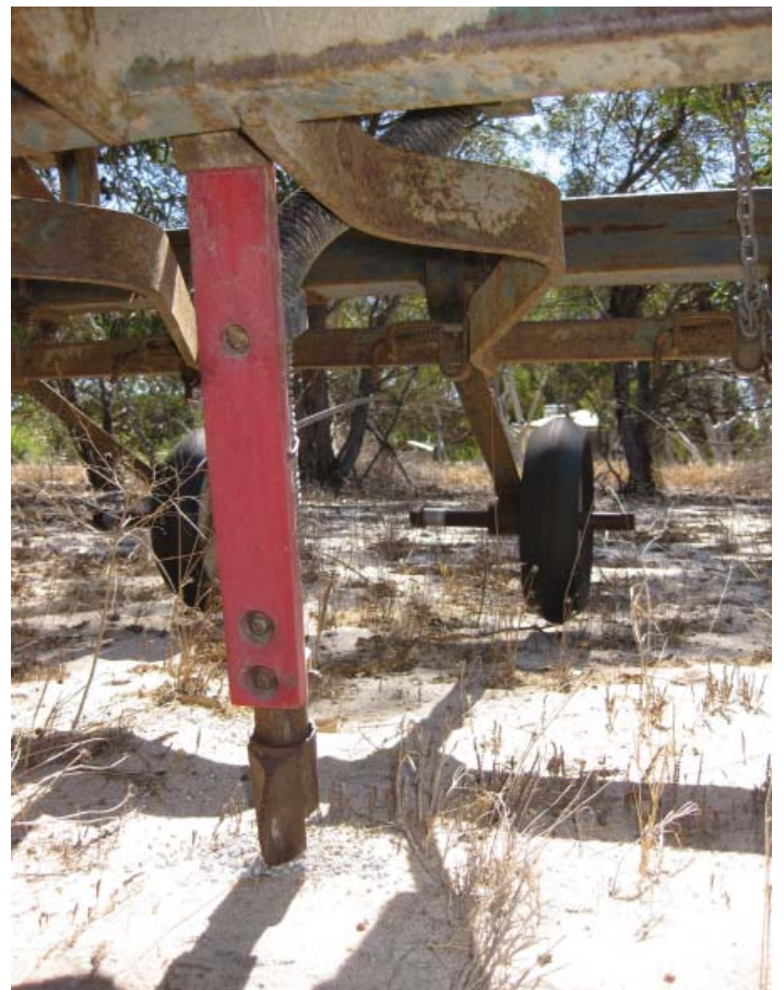
Part of the undercarriage of the converted combine Jim uses to sow subtropical perennial grasses
