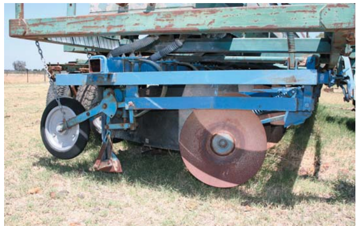
Fig 2. Soilrider tynes with press wheels were mounted on a cultitrash undercarriage under the Shearer wide seeder. Chamberlain plough discs were later added to remove the non wetting soil.
